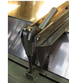
Fast and Easy Screen changes with our Quick-Release Clamps.
